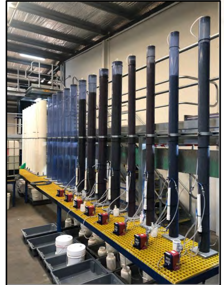
Heap Leach Column Testing
