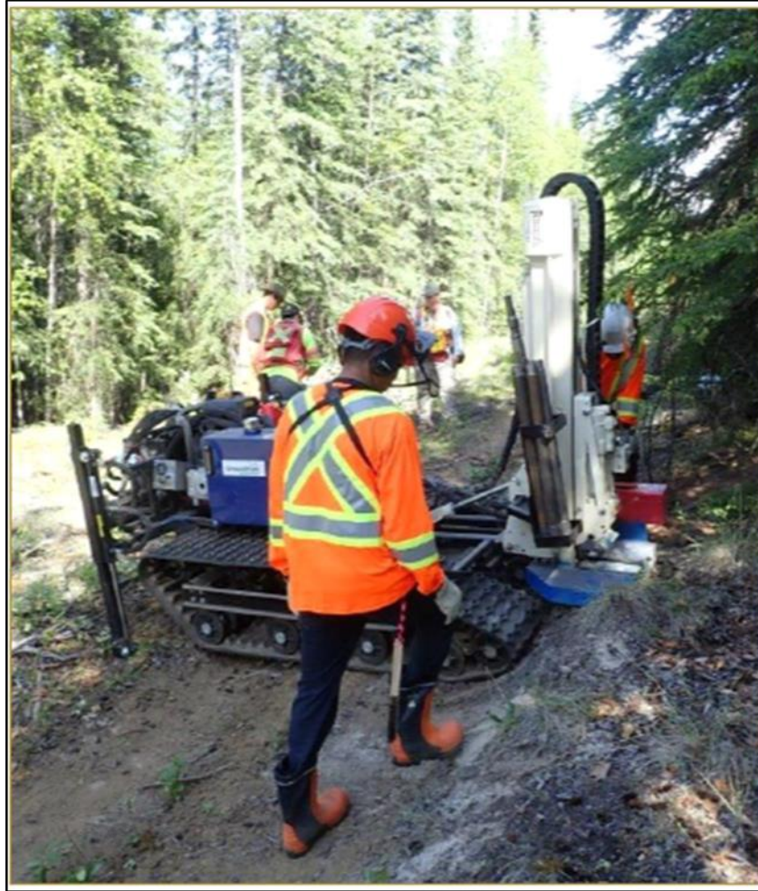
Figure 54: Geoprobe in operation (Tectonic Metals Inc. after Ground Truth Exploration Inc.)
